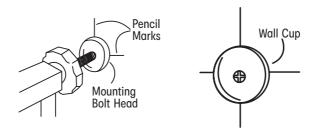
4. Place the gate in opening and ensure the bottom rail is completely flat on the floor and the wall cups are directly above each other, mark the position of each mounting cup, stick the cups in position with adhesive pads.
