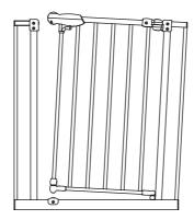
2. When you unpack the gate you may notice a gap at the gate opening, this is normal with pressure mounted gates and the gap will disappear when it is installed correctly.
