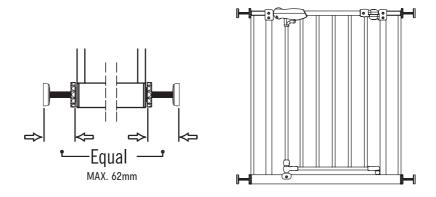
5. Align gate with wall cups and tighten adjuster screws by turning clockwise, starting with the bottom and then the top.
